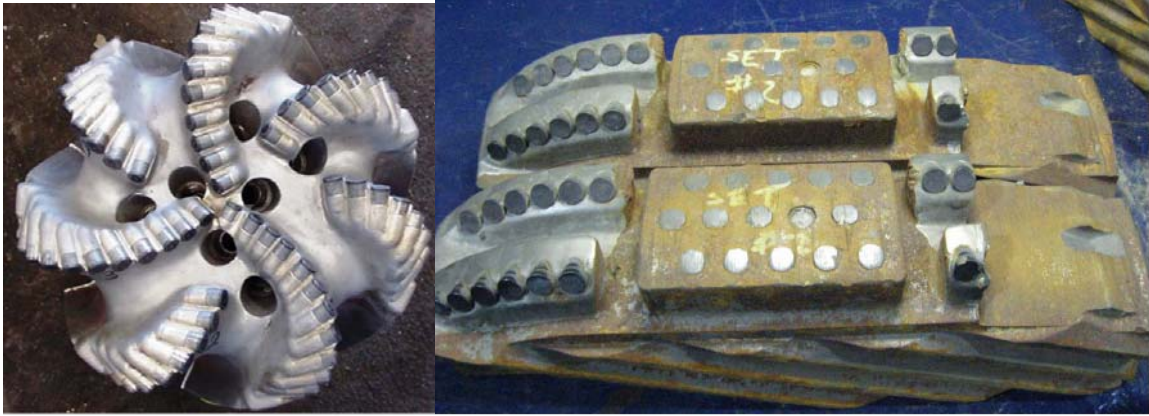
Figure 4 – Dull photos of 7-bladed PDC bit and damaged reamer from WELL #2. Note the reamer’s lower cutter block is substantial worn away and is missing 11 of its 14 original PDC cutters.
