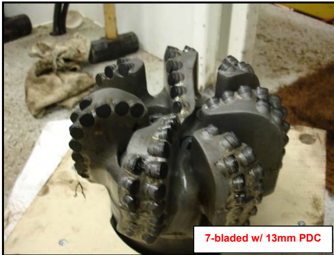
Figure 5. The less aggressive PDC bit used in the above run. This picture was taken after the above run.
