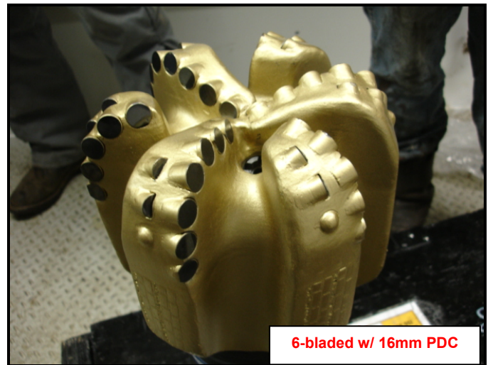
Figure 7. The more aggressive PDC bit used in the above run. This picture was taken before the above run.
