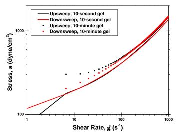
Figure 3 Thixotropic loop at 120°F for Fluid #2, performed after 10-second and 10-minute gel periods, demonstrating the strong thixotropic nature of the drilling fluid.
