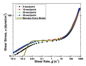
**Figure 13** Controlled stress flow curves at 120°F, with varying equilibration times for each data point, for Fluid #4, demonstrating behavior similar to that predicted by the Mendes-Dutra model.
