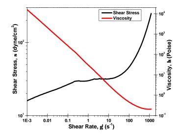
**Figure 9** Controlled rate flow curve at 120°F for Fluid #4, demonstrating behavior similar to that predicted by the Mendes-Dutra model.
