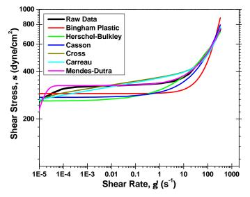
**Figure 14** Controlled stress curve at 120°F for Fluid #2, at 100-seconds per data point, with fits from the standard models and the Mendes-Dutra model.
