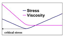
Figure 2 Shear stress and viscosity as a function of strain rate as predicted by Equation 4, for n=2. Illustrated is the critical stress below which flow is unstable.
