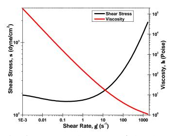
**Figure 8** Controlled rate flow curve at 120°F for Fluid #2, demonstrating a behavior similar to that predicted by the thixotropy model for a fluid with a strong structural growth component.
