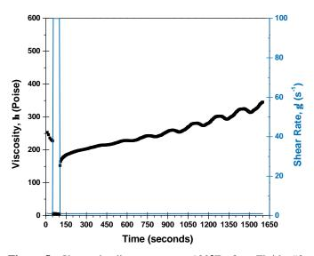
Figure 5 Shear loading test at 120°F for Fluid #2, demonstrating the steady growth of structure under shear.
