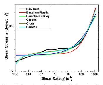
Figure 11 Comparison of standard model fits to the flow curve for Fluid #4, from controlled rate testing at 120°F.
