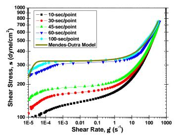
**Figure 12** Controlled stress flow curves at 120°F, with varying equilibration times for each data point, for Fluid #2, demonstrating behavior similar to that predicted by the Mendes-Dutra model.
