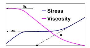
Figure 1 Shear stress and viscosity as a function of strain rate as predicted by Equation 1, the Mendes-Dutra viscosity function.
