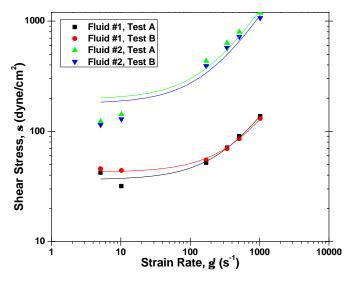
**Figure 6** Viscometry results for Fluids #1 and #2 at 120°F when tested by Test Methods A and B and fit by the Bingham plastic model using only the 600-rpm and 300-rpm data.
