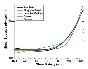
Figure 10 Comparison of standard model fits to the flow curve for Fluid #2, from controlled rate testing at 120°F.
