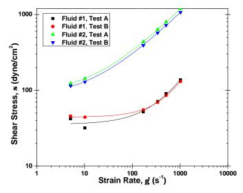
**Figure 7** Viscometry results for Fluids #1 and #2 at 120°F when tested by Test Methods A and B and fit by the Bingham plastic model using all six data points.
