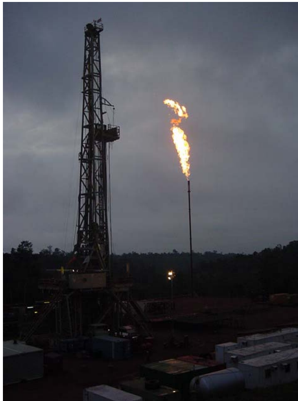
Fig. 1— Field case showing gas flared during the UBD operation.
