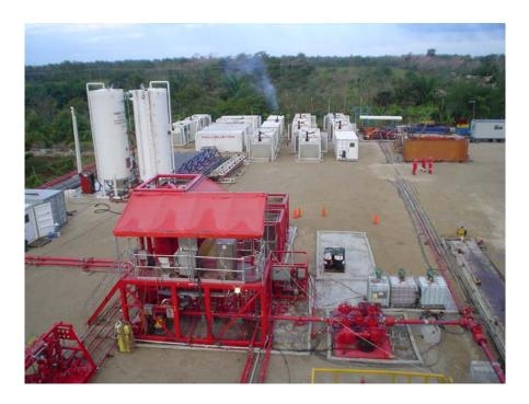
Figure 3 — Equipment rigged up at location for MPD onshore field case.
