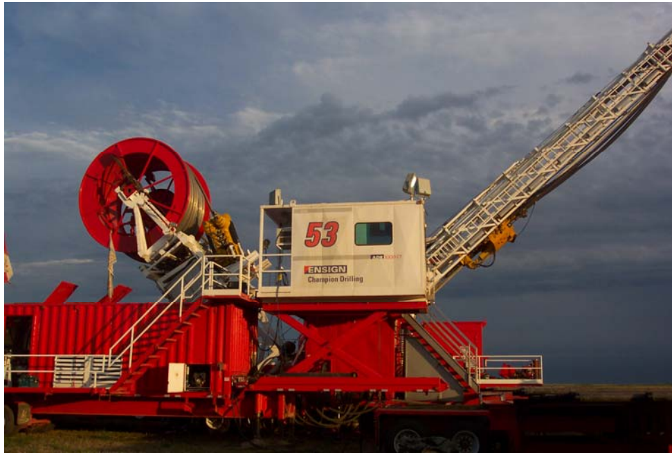
Figure 2: Hybrid Rig Transition from Conventional Drilling to Coil Drilling
