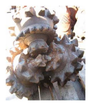
Figure 19 – 17-1/2" HVST dull in good condition after 4978' of drilling, the dull grade was 1 2 WT G E I ER HR.
