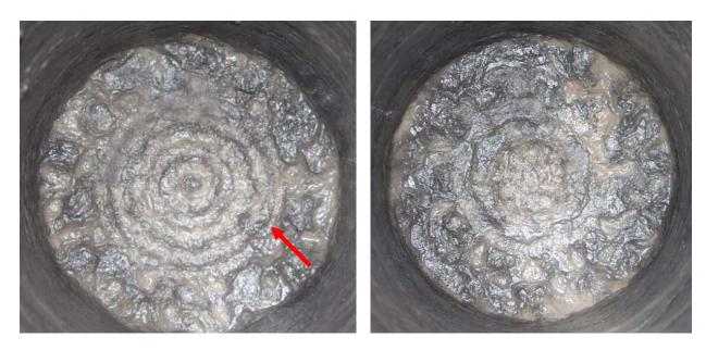
Figure 8 – Laboratory bottomhole patterns for the 9-7/8" HVST bit (left) and the standard 117 bit (right). The arrow in the left photograph identifies the kerf being drilled by the HVST bit's anti-tracking row.
