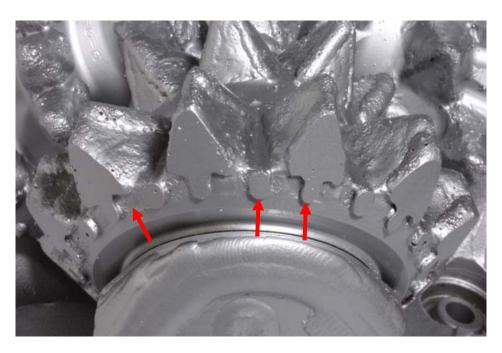
Figure 11 – Welded gauge trimmer pads, or bar trimmers, shown by two vertical arrows. Note the continuous ring of hardfacing on the cone gauge surface between the bar trimmers, shown by the inclined arrow.
