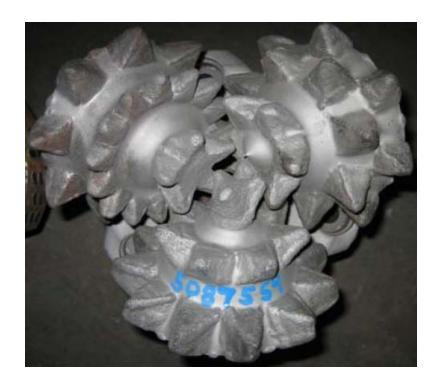
Figure 15 - 9-7/8" HVST bit run #2 which achieved 74 fph section ROP. The dull is in excellent condition after 4392' of drilling with a dull grade was 1 1 WT A E I CT TD.
