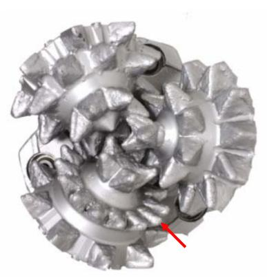
Figure 5 – Bottomhole view of the new 9-7/8" HVST bit. Note the anti-tracking row identified by the arrow.
