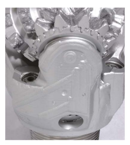
Figure 13 – Improved shirttail and leg hardfacing on 12-1/4" HVST bit reduces the damaging effects of hole-wall contact.
