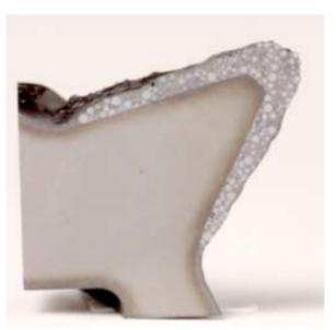
Figure 6 – Cross-section view of a Pyramid inner row tooth. Note the thick hardfacing deposit on the tooth crest.
