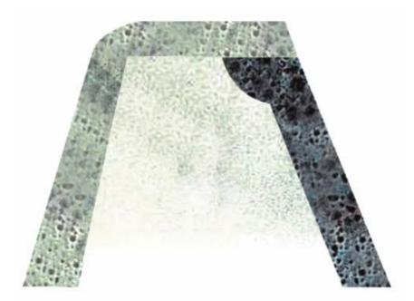
Figure 10 – Cross-section of a heel row tooth with bi-metallic gauge for wear resistance and tooth durability. The darker hardfacing is on the ground gauge surface.
