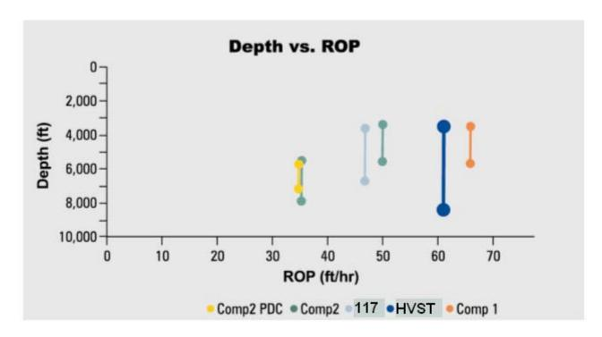
Figure 16 - 12-1/4" Bit run comparison of one HVST bit run vs several competitor tricone 117 ST bit offsets and one competitor PDC bit offset. The HVST bit more than doubled the footage of the best offset, and drilled faster than all the offsets that approached this depth range.
