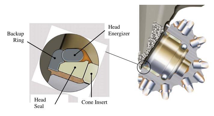
Figure 12 – Second generation single energizer metal seal bearing (SEMS2) with enlarged view of seal package (circa 2005).
