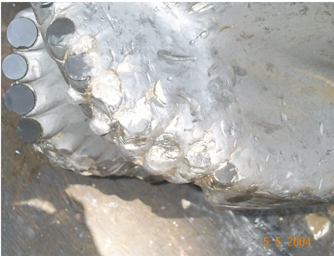
Fig. 20—Close-up of bit damage occurring with no S&V mitigation.
