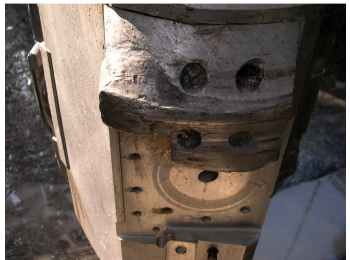
Fig. 21—Failure due to improper bit selection and lack of mitigation process in place.
