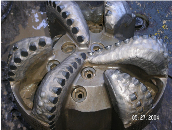
Fig. 22—This bit was recommended after the pre-drill analysis. The bit drilled the section without incurring any damage and was graded as new.
