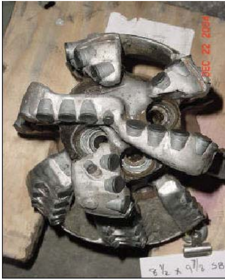
Figure 1 – Bicenter bit used in conjunction with point-the-bit technology
