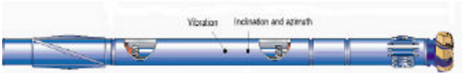
Figure 5. Fully-rotating rotary steerable system used in this case study. Features no external non-rotating parts and provides automated directional control in vertical well applications.
