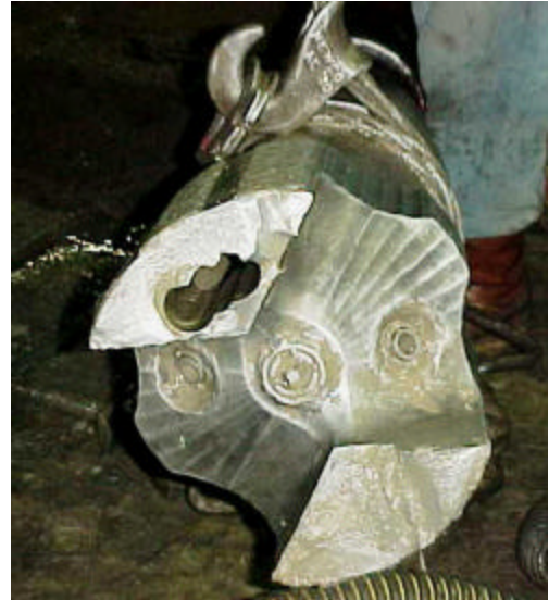
Figure (4) – Flip Arm Broken in Half
