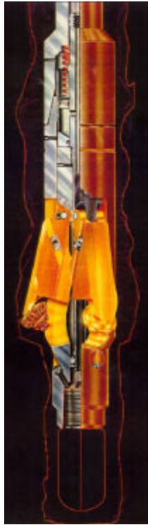
Figure (3) – Hydraulic Activated Flip Arm Underreamer
