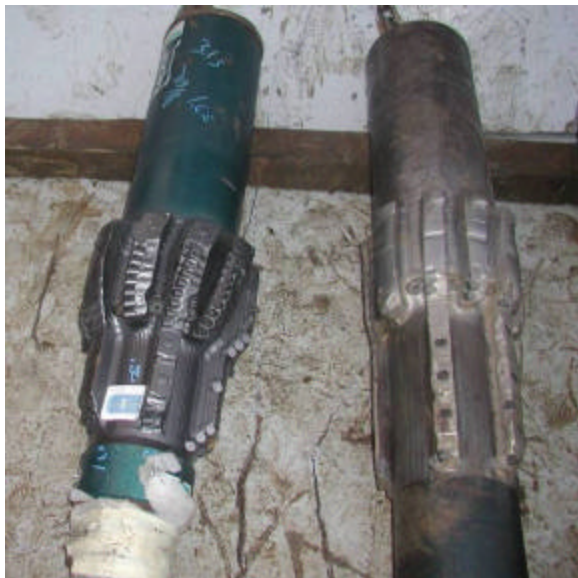
Figure (5) – Bi-Center / Winged Reamer – New versus Used
