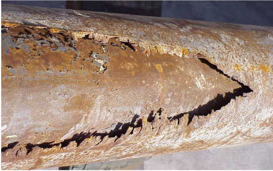
Figure 3 – Inadequate window conditioning. Jagged edges create the potential for severe damage to the solid expandable tubulars.
