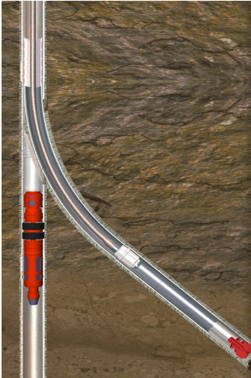
Figure 1 – Example of solid expandable tubular deployment in conjunction with whipstock technology.
