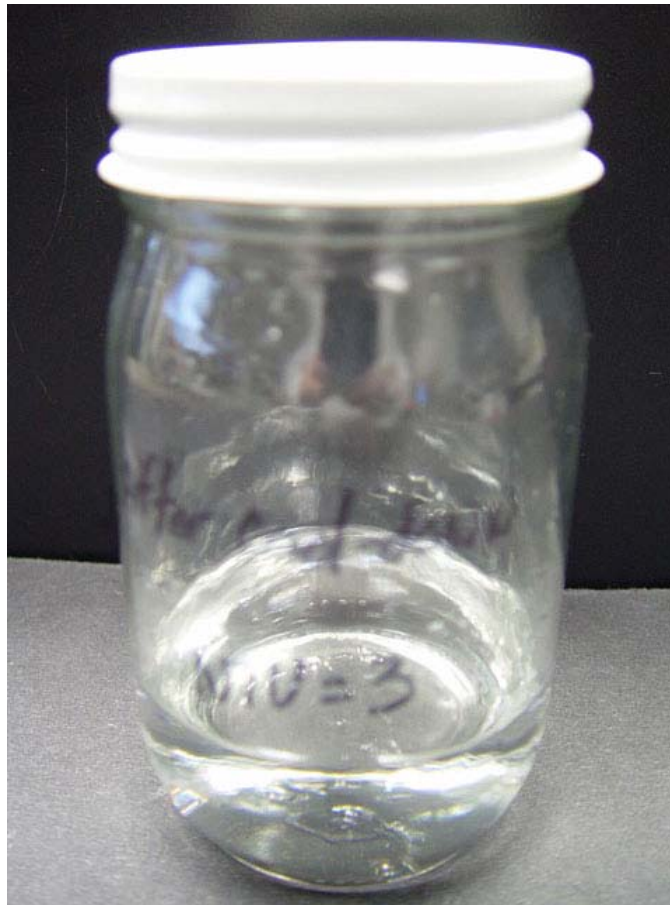
Fig. 8 – Digital images of a compatibility test of a 13.7-lb/gal NaBr/CaBr 2 blend. This blend was heated to 300°F for 6 hours and then cooled rapidly. Turbidity after cooling was approximately 3 NTU.
