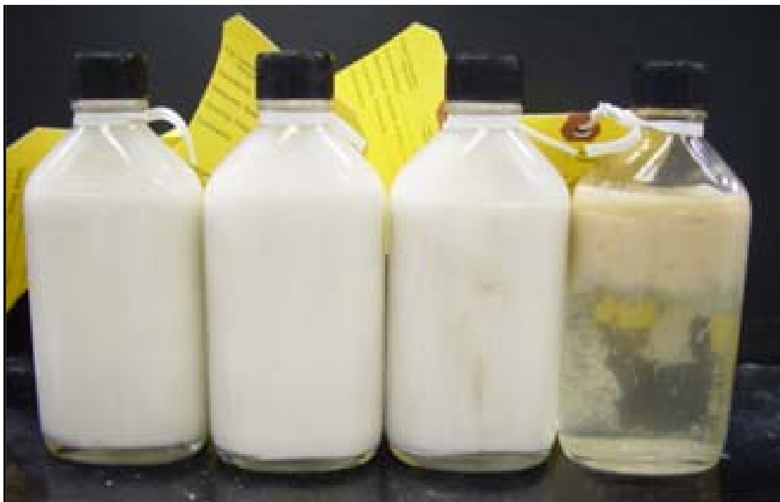
Fig. 14 – Produced fluid sample (right-side) from the initial flowing of the well. This sample was collected after stimulation with acid.
