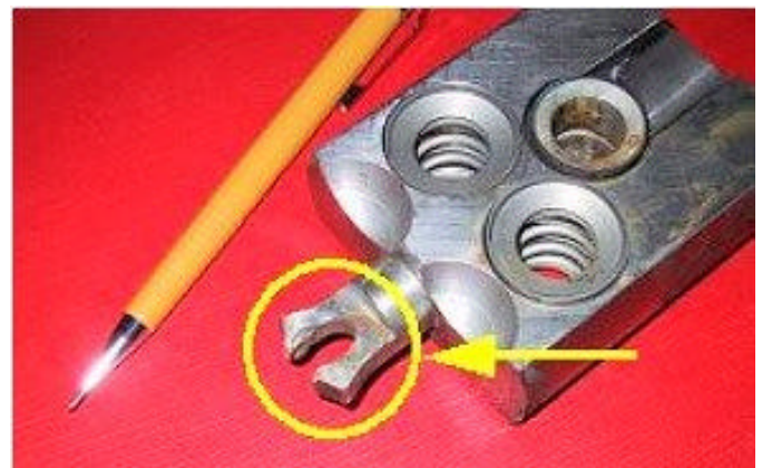
Fig. 4 - Damaged seal carrier from the 5K to 3K manual regulators. The regulator is from the HP shear ram circuit.
