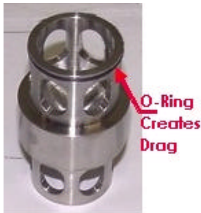
Fig. 10 - The piston of the new Gilmore HDHI shuttle valve. The arrow points to the O-ring that provides the drag when the valve changes direction.
