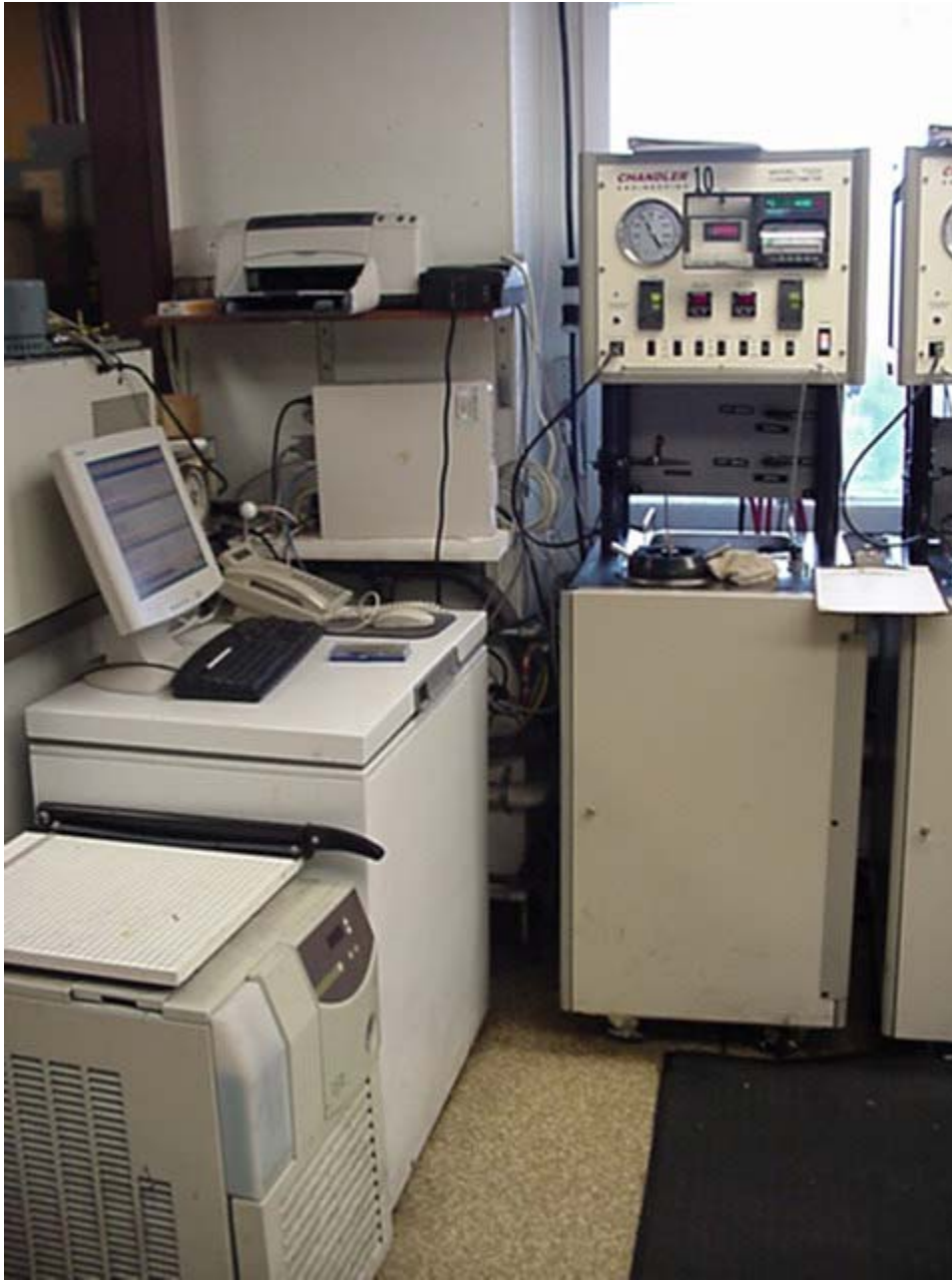
Fig. 3—Consistometer equipped with chiller.
