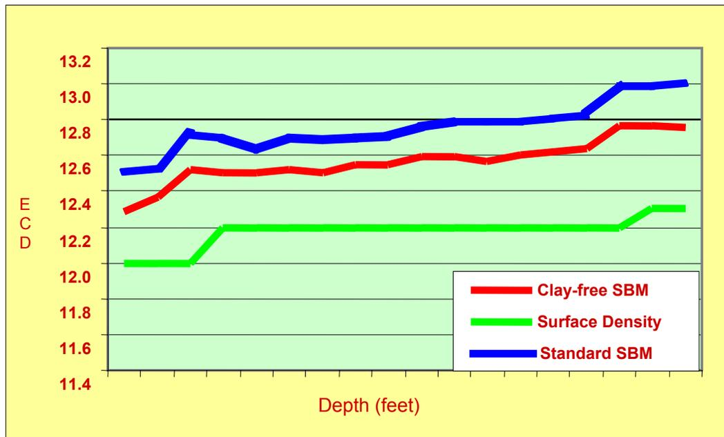
Figure 2: ECD in ppg of the clay-free synthetic base mud, using a downhole pressure measurement tool, compared with that of a conventional SBM used on a nearby offset well in deepwater Gulf of Mexico.
