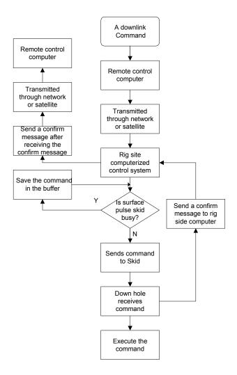
Figure 6. Remote Control Flow Chart
