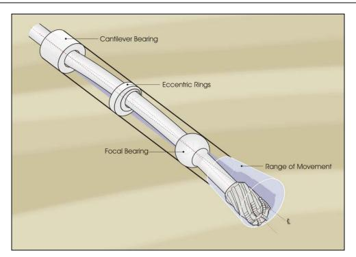
Fig 3. A points to Bit Rotary Steerable Tool Concept (Cited from Tetsuo, et al. [1])
