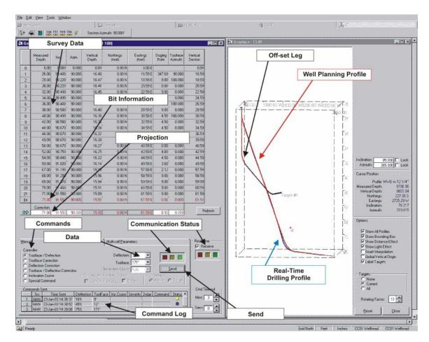
Fig 5. Downlink Drilling Control and Survey Data Display
