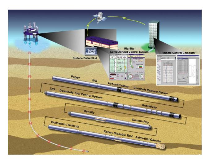
Figure 1. Downlink Drilling Control System and Downhole BHA Integration (adapted from Tetsuo, et al. [1])
