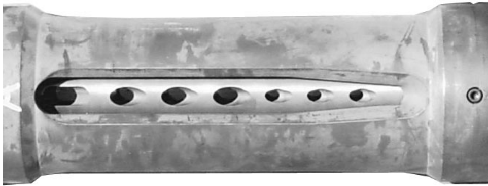
Fig. 5 — Crossover Prior to Test 1: 50 bbl/min test
