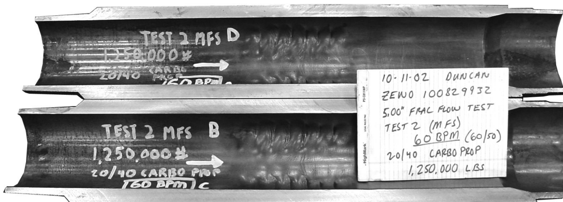
Fig. 19 — Upper Extension Erosion Pattern at Crossover After 1,250,000 lbm, Test 2 Run 4, End of 60 bbl/min Test
