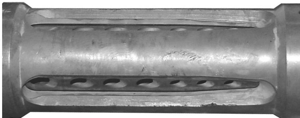
Fig. 17 — Crossover Prior to Test 2: 60 bbl/min Test
