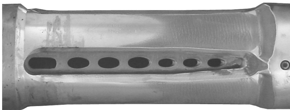
Fig. 18 — Crossover After 1,250,000-lbm, Test 2 Run 4, End of 60 bbl/min Test
