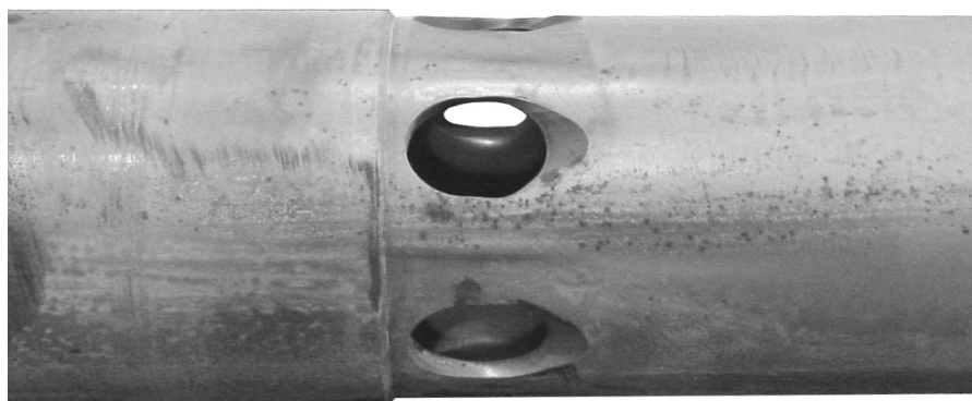
Fig. 14 — Closing Sleeve Housing After 2,003,700 lbm, Test 1 Run 6, End of 50 bbl/min Test
