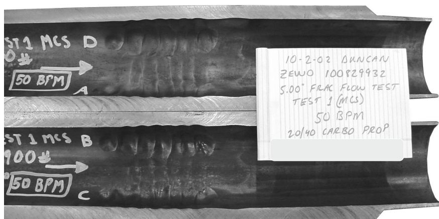
Fig. 15 — Upper Extension Erosion Pattern at Crossover after 2,003,700 lbm, Test 1 Run 6, End of 50 bbl/min Test
