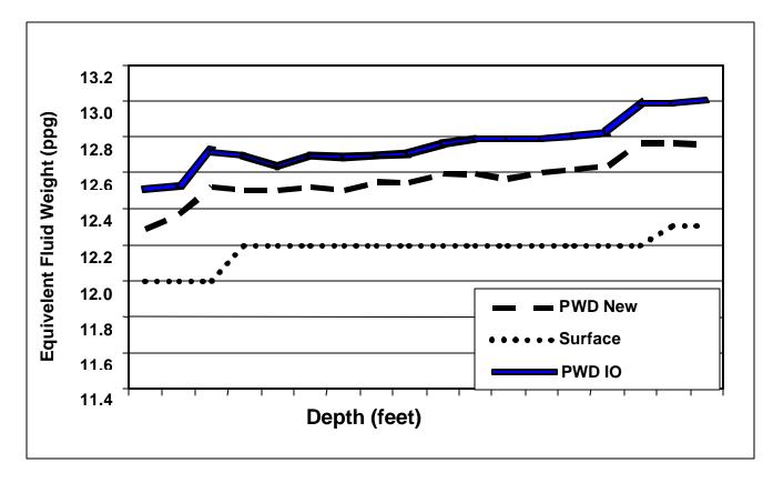
Figure 1 The New System: ECD Comparison
