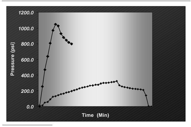
Figure 3. The before (lower curve) and after(upper curve) treatment LOT results for a deep HPHT well drilled with SBM
