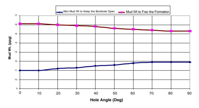
Figure 2. Example output from a linear-elastic borehole stability model showing the minimum and maximum mud weight predictions.
