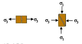
Figure 1 Rock Failure: Tensile (left) and Compressional or shear (right)
