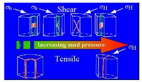
**Figure 2 Modes of failure.** Shear failure from left to right: wide breakout, shallow knock out, high angle echelon and narrow breakout. Tensile failure: circumferential failure and fracturing.
