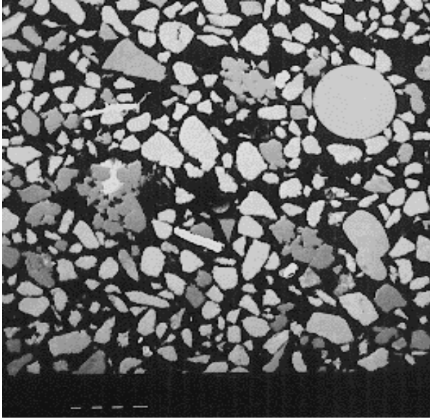
Fig. 5a – SEM-BSE image of drill cuttings sample from field Example A. Note different textures and gray tones. The last segmented bar scale (left) represents 100 microns.
