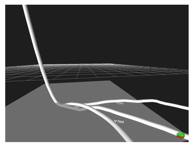
Figure 5. Geometry of ITBS Triple Lateral in Relation to GOC and GWC
