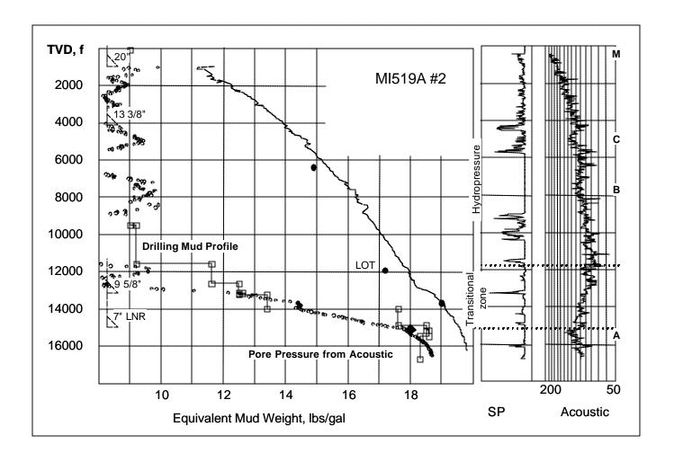
Figure 4. Wel MI519A #2. Long transitional zone – result of pressure seal damage.
