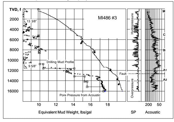
Figure 3. Wel MI486 #3. Two pressure compartments separated with fault.
