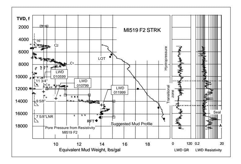
Figure 5. Wel MI519 F2 sidetrack. Real-time pore pressure analysis using LWD alow to optimize casing program in long transition zone (damaged seal).
