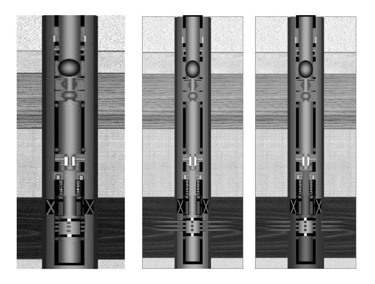
Fig. 3 — Annulus pressure is applied to activate the firing head and open top and bottom flow vents, allowing junk and mud to go to the lower chamber. Fig. 4 — Perforating.
