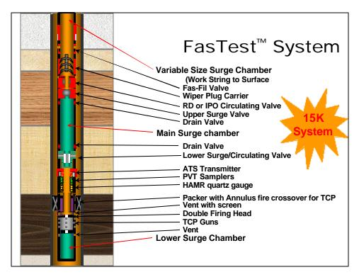
Fig. 2 - Configuration of the system.
