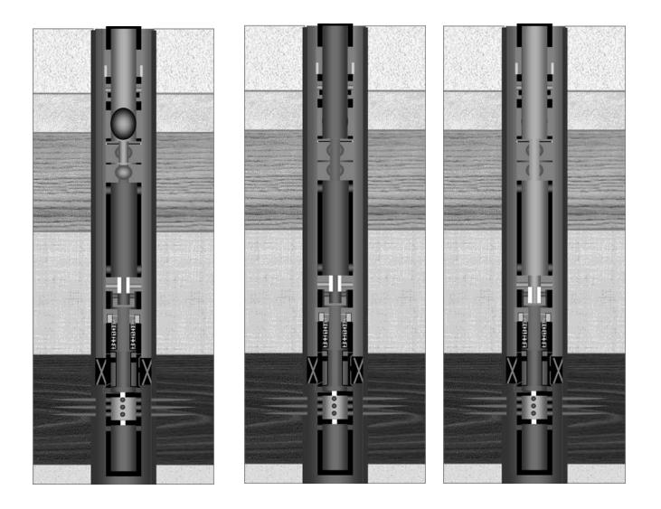
Fig. 6 — Annulus pressure is reapplied to shift the lower surge/circulating valve to the well test position, starting the second surge and shut in period. Fig. 7 — Annulus pressure is reapplied to open the upper surge valve, starting the third surge/flow period. Well is circulated, and a large volume sample is recovered at surface. Fig. 8 — Circulating the well.
