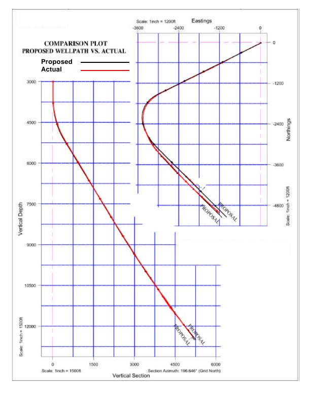
Figure 2 – Planned versus actual well profile for well in Ship Shoal.
