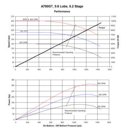
Fig. 4- Power Curve for the A700GT5:6 motor
