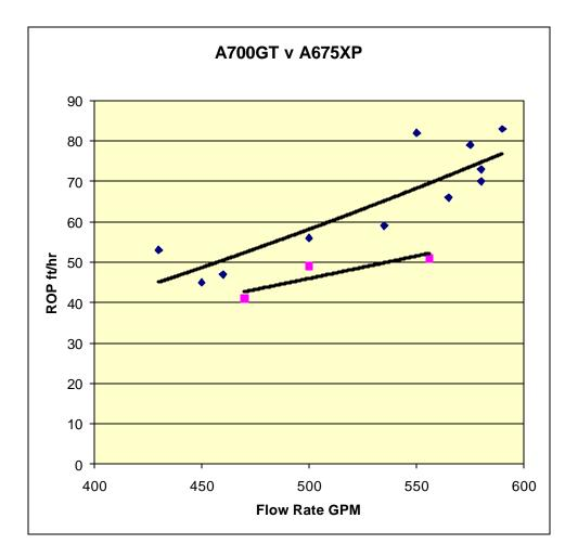
Fig. 5 ROP vs flow rate
