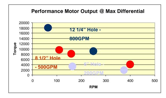
Fig. 2- Performance motor output.
