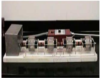
Fig 8 – The Slake durability tester.
