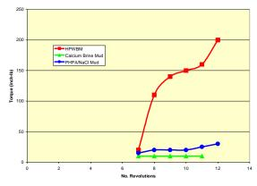
Fig 4 – Bulk hardness test comparing the torque readings on Arne Clay cuttings from three inhibitive systems.
