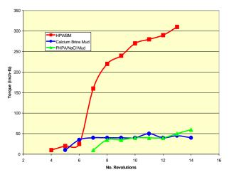
Fig. 5 – Bulk Hardness test comparing the torque readings on Oxford Clay cuttings from three inhibitive systems.
