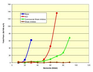
Fig. 2 –Bentonite inhibition test comparing the yield point of three shale inhibitors and the base fluid.
