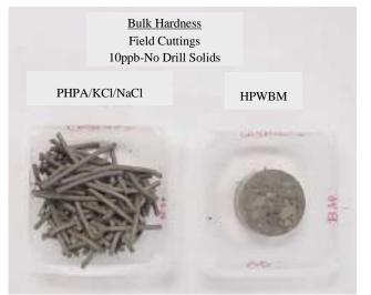
Fig 7a – Field cuttings exposed to inhibitive fluid and then extruded using the Bulk Hardness procedure.
