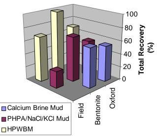
Fig. 9 – Comparison of three types of clay cuttings exposed to various inhibitive muds as measured by percentage of cuttings recovery using the Slake durability test.
