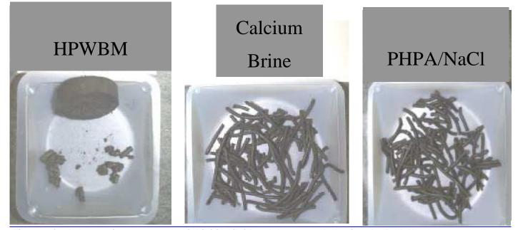
Fig. 6 Oxford clay cuttings exposed to inhibitive fluid and then extruded using the Bulk Hardness procedure.
