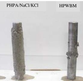
Fig 10e – Accretion tests using two inhibitive muds and field cuttings from the Gulf of Mexico.
