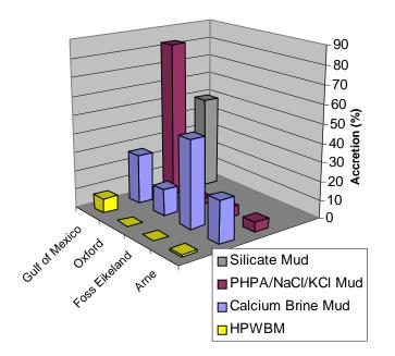
Fig. 11 – Comparison of four types of clay cuttings exposed to various inhibitive muds as measured by the percentage accretion.
