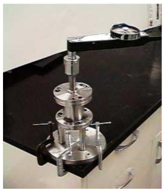
Fig 3 – Bulk hardness tester.
