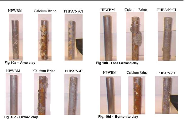
Fig. 10a-d – Accretion tests using three different inhibitive muds (HPWBM, Calcium brine, PHPA/NaCl mud) and four different clays (10a – Arne, 10b- Foss Eikeland, 10c – Oxford, 10d – bentonite clay).
