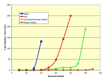
Fig. 1 – Bentonite inhibition test comparing the 3 rpm Fann readings of three shale inhibitors and the base fluid.
