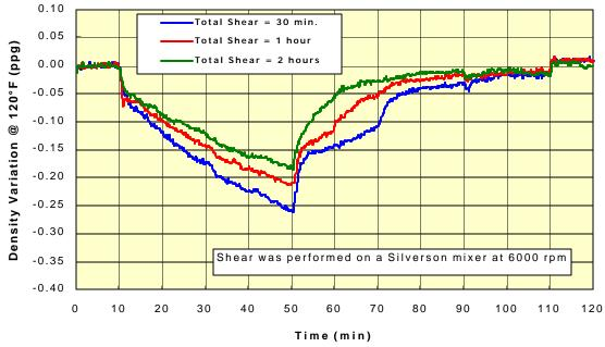
Fig. 4 – Density variation curves with 2-lbm/bbl treatment of organophilic clay and three stages of shearing with a 14.3-lb/gal SBM.
