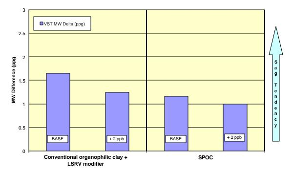
Fig. 1 – Effect of organophilic clays on sag tendency measured by VST in laboratory fluids.
