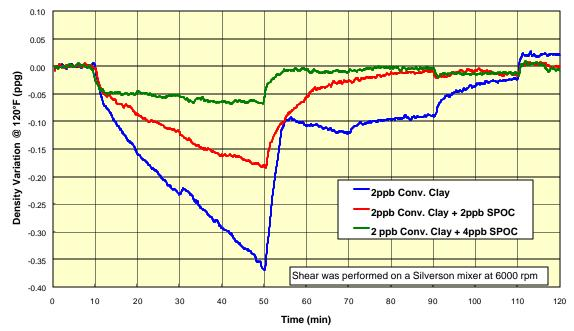
Fig. 7 – Effect of SPOC addition to 14.3-lb/gal SBM illustrated by SFLT density variation curves.
