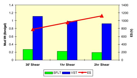
Fig. 5 – Effect of shear on SFLT, VST and ES results.
