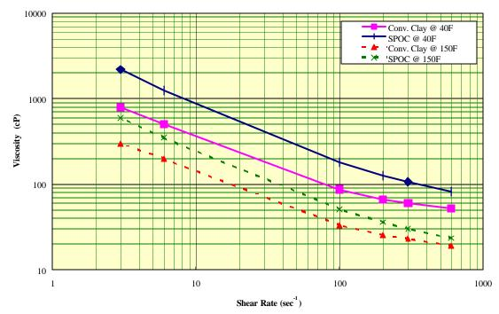
Fig. 3 – Effect of 4-lb/bbl organophilic clays on rheology of SBM at different temperatures.
