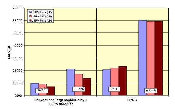
Fig. 2 – Effect of organophilic clays on Brookfield LSRV in laboratory fluids.
