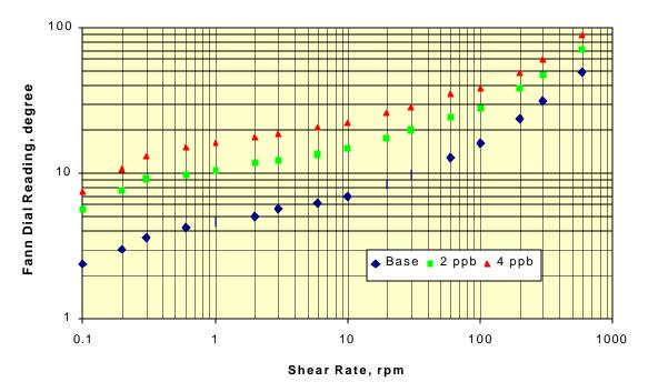
Fig. 8 – Effect of organophilic clay content on rheology of 14.3-lb/gal SBM sheared for 2 hours.
