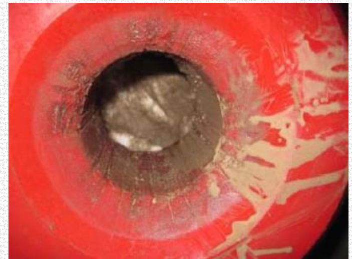
After 60 passes with a 4” protector @ 700 psi.
