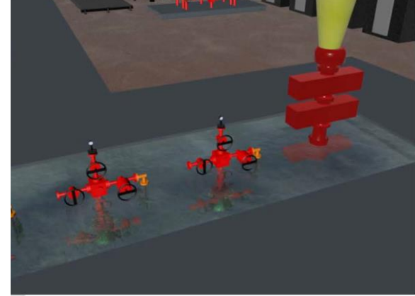
Wellhead Design With Two (2) Submerged Valves. Pneumatic Valve Located Above Ground Level.
