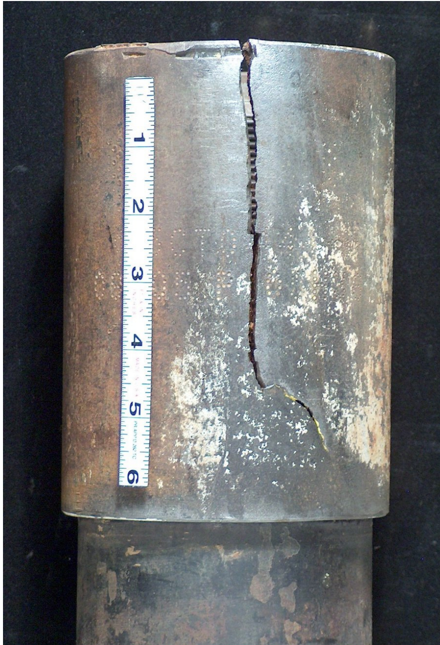
Figure 7 Grade P110 coupling failure that initiated at mechanical damage, shown at the top.
