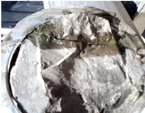
Natural fracture stained with oil (core depth at 6873 ft)
