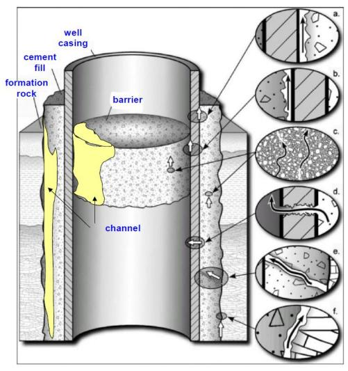
Interface casing/cement (micro-annulus, channel)
