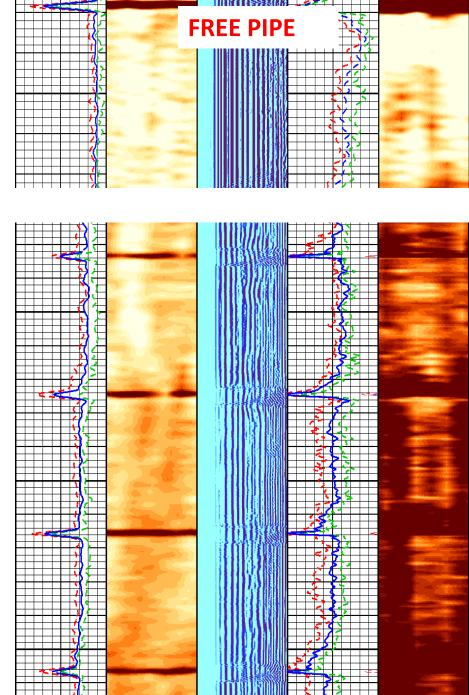
Channel detection in Production / Injection wells
