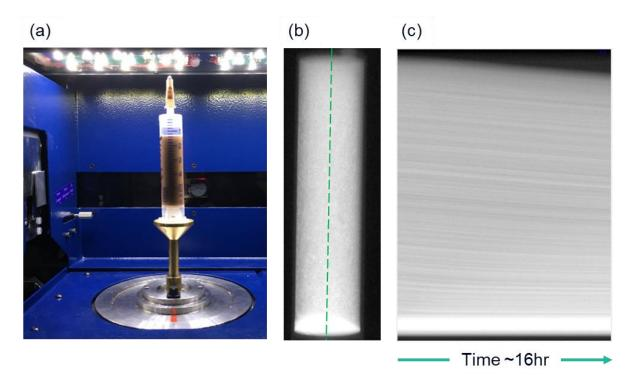
Figure 1 – Model drilling fluid sample, constructed to show rapid syneresis, in a standard 5ml syringe. (a) sample mounted in a syringe tube within the x-ray microtomograph instrument (Bruker, SkyScan 1275 micro-CT scanner) (b) shadowgraph image taken at start of experiment (white is dense barite) showing initial distribution of barite particles. (c) time evolution of centerline of image (b) as indicated.
