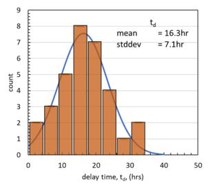
Figure 6 – Thirty-two identical drilling fluid samples were allowed to stand quiescently. The gel interface height was measured optically and each individually followed the behavior illustrated in Figure 2. Plotted here is a histogram of the observed delay time before free oil was observed.
