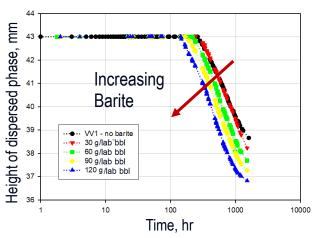
Figure 2 – Height of interface of model OBM gel with supernatant as a function of time for several barite loadings measured using a Turbiscan (Formulaction) instrument. Initially there is no free oil. Free oil appears for this formulation after about 110hr. Subsequently the height of the gel phase drops in an exponential fashion.
