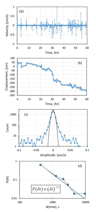
Figure 4 – Speckle velocimetry of a model drilling fluid gel collapse (a) velocimetry as a function of time, intermittent high velocity events are observed rather than steady settling, (b) integration of the velocity for displacement, (c) probability distribution function of the data in (a), and (d) probability distribution of times between events.
