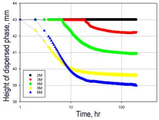
Figure 3 – Height of interface of model OBM gel with supernatant as a function of time for varying brine salinity. The delay time is minimized at the minimal Van der Waals interaction strength (5M).
