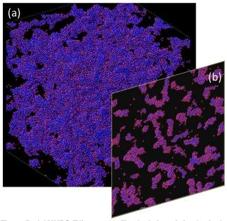
Figure 5 – LAMMPS (Plimpton 1995) calculation of simple single component attractive system having undergone arrested phase separation. Initial volume fraction 0.2. The particles cluster forming a system spanning 3D network of glassy strands. (a) a projection of the 3D computational cell with periodic boundary conditions, (b) a single slice from the same calculation illustrating the clusters more clearly; in 3D these are fully connected.
