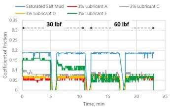
Figure 8: Lubricity of 14.0 ppg saturated salt mud on steel-shale contact measured with the LEM.
