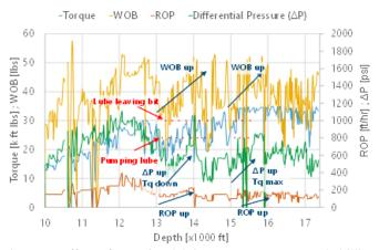
Figure 9: Effect of pumping lubricant sweeps on several drilling parameters.
