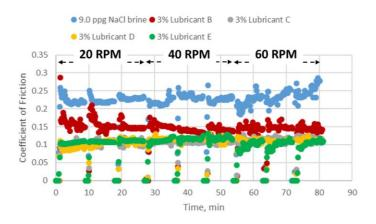
Figure 2: Lubricity of 9.0 ppg NaCl brine on steel-shale contact measured with the dynamic lubricity tester.
