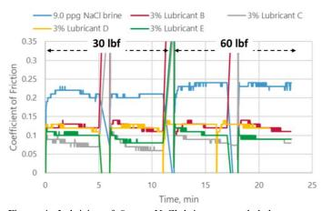
Figure 4: Lubricity of 9 ppg NaCl brine on steel-shale contact measured with the LEM.
