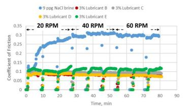
Figure 1: Lubricity of 9.0 ppg NaCl brine on steel-steel contact measured with the dynamic lubricity tester.
