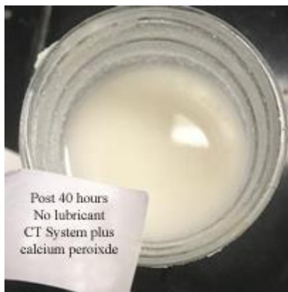
Figure 15 – Phase II, Post 40 hours. Figure 15A (left) shows the CT system plus lubricant and Ca-peroxide. Greasing is ubiquitous as adheres to the side of the jar. Figure 15B (right) shows the CT System with calcium peroxide suspension however no lubricant was incorporated.
