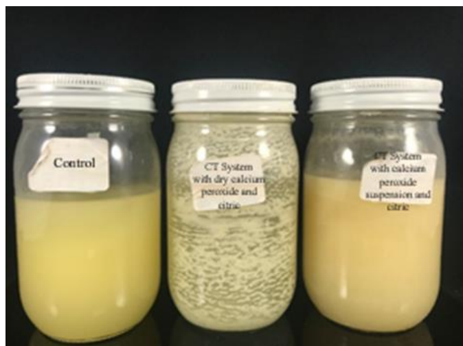
Figure 12 – Post 40 hours: Left to right: Control, calcium peroxide suspension, and dry peroxide in suspension with 0.25-lb/bbl citric acid. Note formation of grease.
