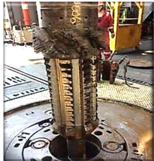
Figure 14 – Brush/Magnet WBCU tool post run
