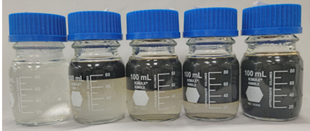
Digital image showing test jars, 3% KCl with NE1, after 30 minutes of static aging at 150°F
