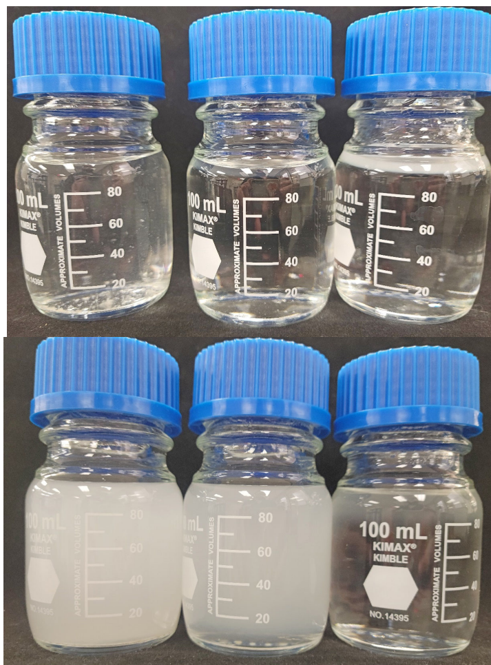
Figure 4 – Digital images showing 2% w/w KCl, 26% w/w NaCl, and 32% w/w \text{CaCl}_2 after the addition of 0.75% v/v NE1 (top). As NE1 is formulated for less dense brines, complete solubility is evident in the two monovalent brines on the left while incomplete solubility is evident upon addition to the \text{CaCl}_2 (thin white layer - jar on right). NE2 (bottom) which is formulated for higher density brines, is shown in the same three brines however more complete solubility is evident in the 32% \text{CaCl}_2 .
