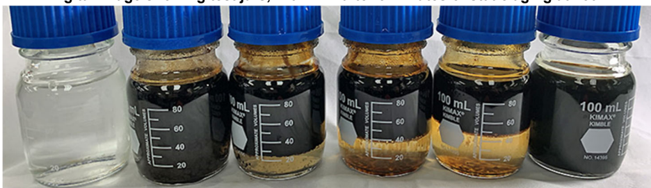
Digital image showing test jars, with NE2, after 15 minutes of static aging at 150°F
