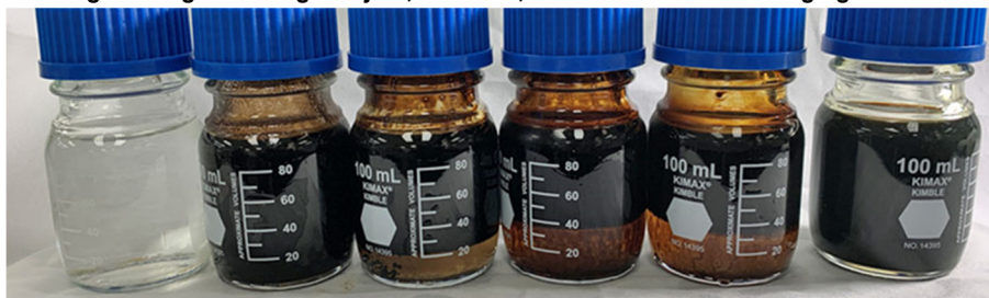
Digital image showing test jars, with NE2 after 5 minutes of static aging at 150°F
