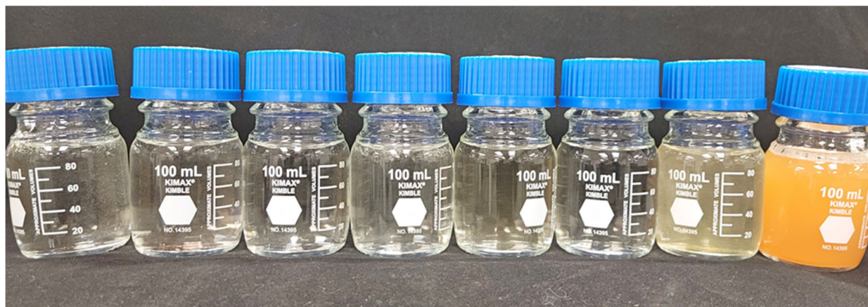
Figure 3 – Digital image showing synthetic brines as described in Table 3, left to right, Brine A, B, C, D, E, F, G, and L, after addition of IC1 at a concentration of 1 gal/1000 gal brine.
