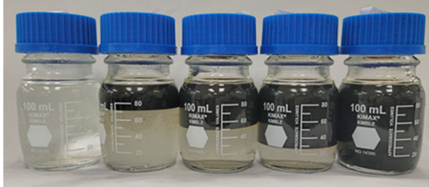
Digital image showing test jars, 3% KCl with NE1, after 5 minutes of static aging at 150°F
