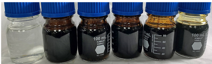
Digital image showing test jars, with NE2, immediately after agitating
