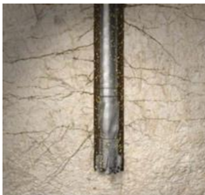
Initially, the WST particles are free-floating in the drilling fluid.
