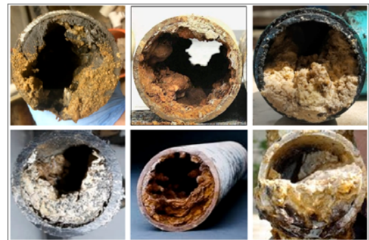
Figure 1. Clogged pipelines in petroleum, mechanical and civil engineering operations – broad ranges in diameters, fluid rheology, debris type and general deposition geometry.
