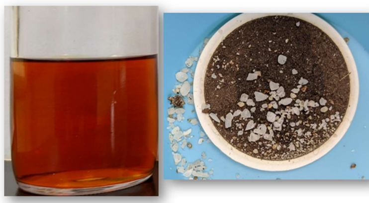
Figure 7 – Acid clean-up test (left: spent fluid; right: residue on disc)
