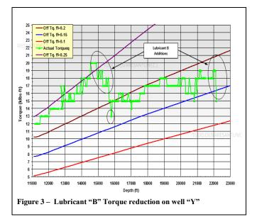
Looking the results on lab and field evaluation was evident the dramatically effect on torque reduction of the Lubricants A & B in IEF.
