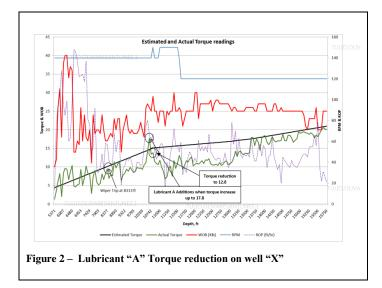
A total of 11,090 ft were drilled horizontally in this well X with lower torque values than estimated after Lubricant A additions.
