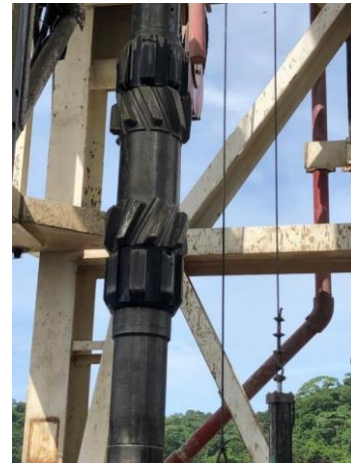
Figure 9 BHA After displacement
