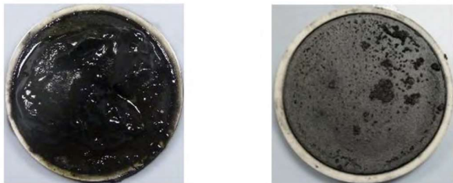
Fig-5 Comparison showing Micronized Ilmenite filtercake before & after acid breaker treatment (OTC-31230)
