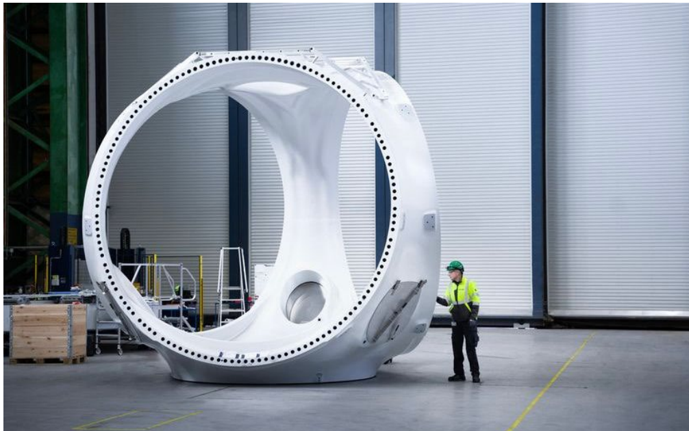
Technician beside the hub of the Vestas 15MW-236m prototype (2022)
