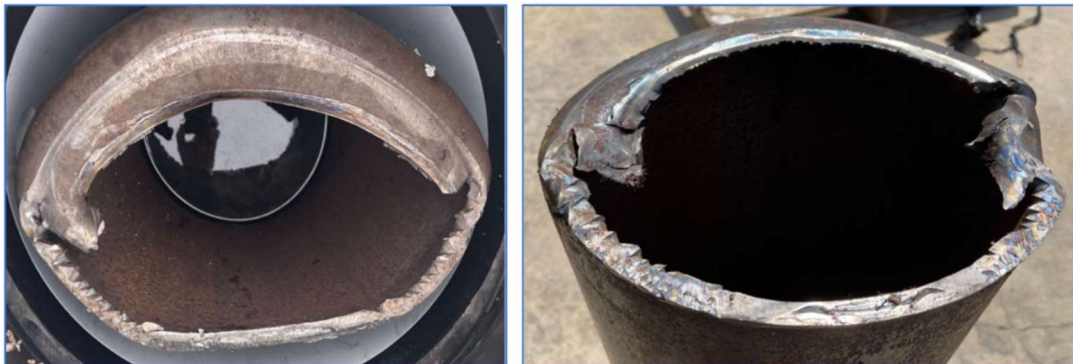
Figure 7: 13-10M K-BOS shear and seal on a 10-3/4" OD Casing, 0.4" WT, P110
