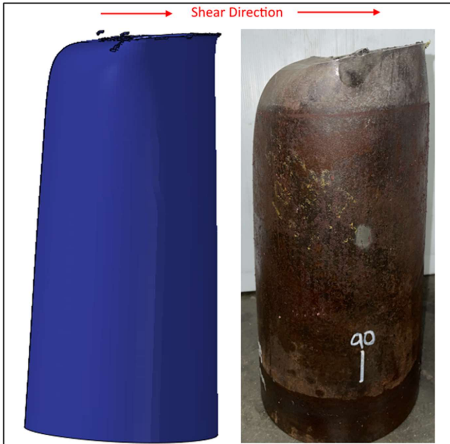
Figure 9: 9-5/8" OD Casing, 0.472" WT, P110 - Model (L) vs. Test Result (R)
