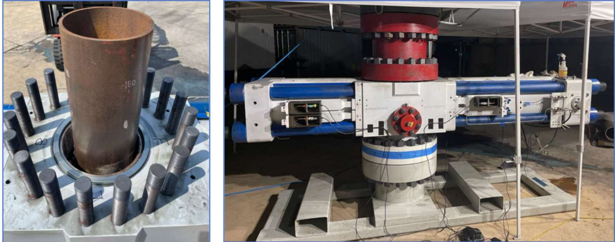
Figure 6: Example of API 16A PR2 shear and seal test set-up for the 13-10M K-BOS
