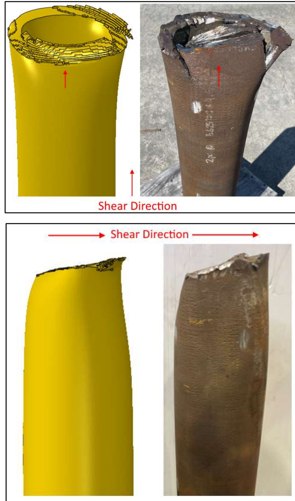
Figure 8: 6-5/8" OD HWDP Landing String, 0.813" WT S135 - Model (L) vs. Test Result (R)
