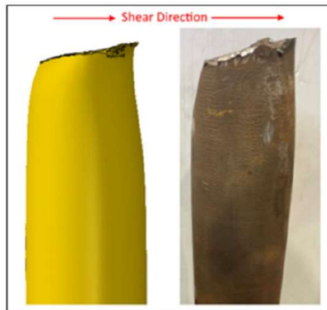
6-5/8" OD HWDP Landing String, 0.813" WT S135 Model (L) vs. Test Result (R)
