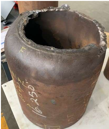
16" OD Casing Q125 136ppf 6-5/8" OD Inner String, V150 50ppf
