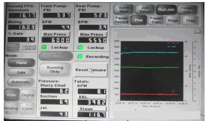
Figure 13: Example of Real Time Data Acquisition on A Cement Pumping Unit
