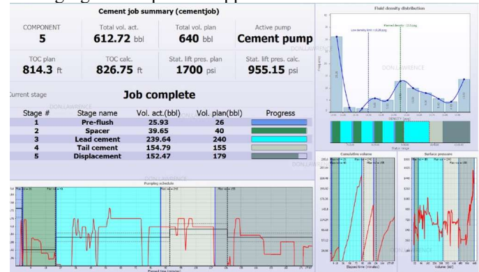
Figure 24: Real Time Cement Evaluation Display from Drilling Rig Data Acquisition Application
