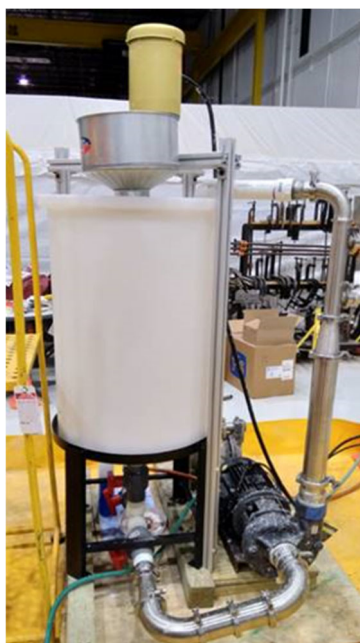
Figure 7 Large-scale batch mixer to replicate field conditions.
