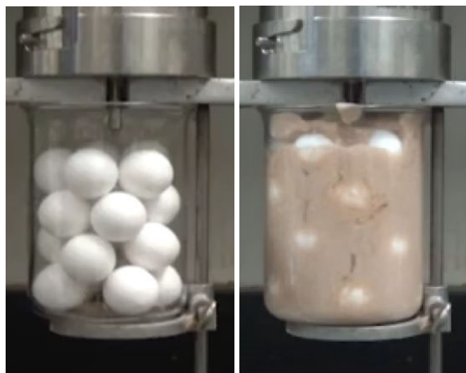
Figure 1 Shear activated cross-linking lost circulation pill showing the ability to fill vugular formations after being sheared through nozzle.
