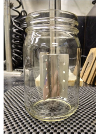
Figure 5 Lab scale mixing in jar with high surface area mixer.
