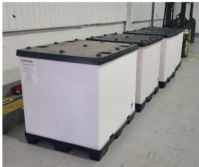
Figure 9 EMS-8650 HT, shear activated cross-linked lost circulation pill packaged in palletized kits.
