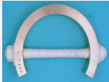
NACE TM0177 Method C C-ring ready to test
